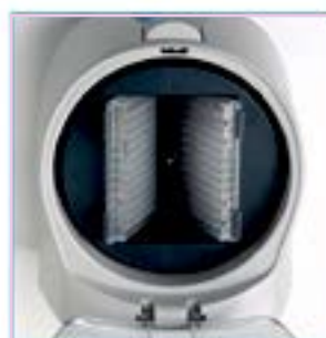
Before & after centrifugation (angled position)
